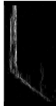
Figure 2. V -disparity space of a road scene: the diagonal bar is the road representation, and the vertical segments are obstacles.
